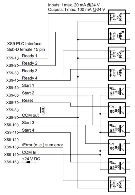
24V DC out should allow 500 mA load
