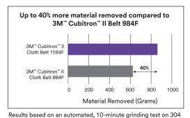
results based on an addinated, forminde grinding test of 304 stainless steel using 36" long belts. Total material removed: the total material removed in grams at 40 cycles.
