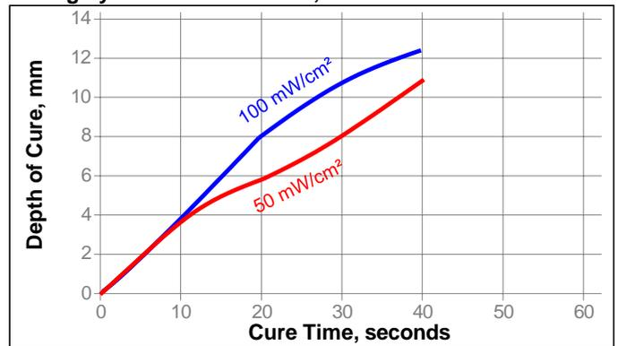
**Curing System: Electrodeless, H bulb**
