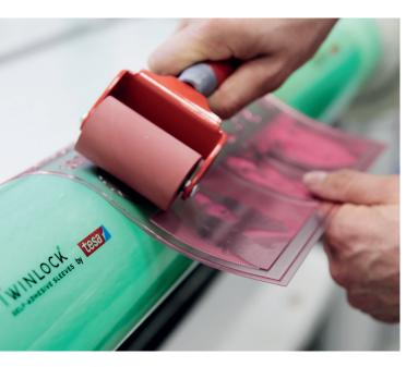
The concept of tesa Twinock® is simple; a self-adhesive and compressible sleeve to mount your flexo printing plates.
